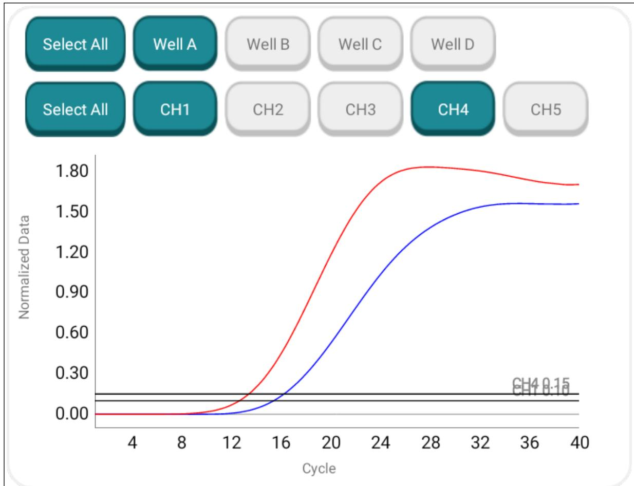
When the Ct value of the sample to be tested is outside the reference range and there is a typical S-shaped amplification curve, the test result is positive;
